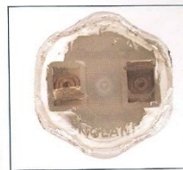
Figure 13.10. Caulk can be used to seal the switch. That used here is of a type which cures clear so that the final switch will not look so messy.
