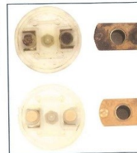
Figure 13.9. A switch as first disassembled (top) and the same switch cleaned (lower).
