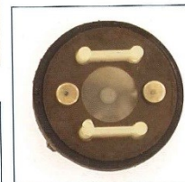
Figure 13.11. The later reverse and overdrive switch had a sealing washer fitted. This example shows the effects of some contact arcing but no corrosion damage.
