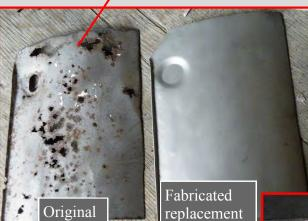
Being a thrifty Scot... fabricating the sheet metal replacements myself for these small sections was a good way to go. Triumph replacement body panels tend to be more expensive than MG.
