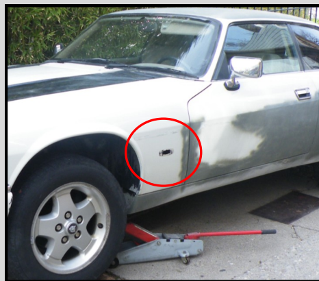
Badges behind the front wheel arches were removed and openings needed to be filled.
