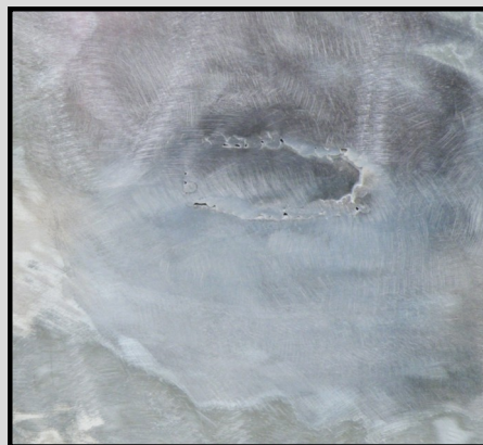
Intermediate grinding of welds to reveal gaps and voids.
