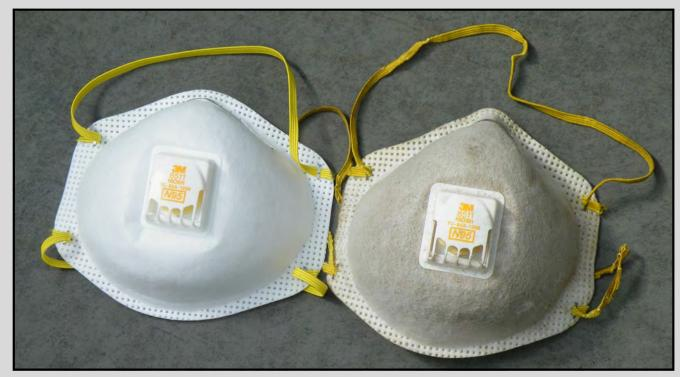
The used respirator on the right shows the effects of less than an hour of use while sanding and grinding. This type of respirator works if you're clean shaven - not good with a beard. Also, if you're painting, a different type of respirator would be needed.
